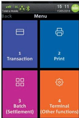
To open the required menu option you can 1. Touch the item on the screen or, 2. Press the item number on the keypad corresponding to the menu item.
